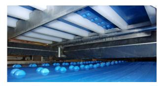
**2) By using the slider bed** Slider bed strips are positioned in such a way that they act as guides for the drive lugs. This means the belt is self-tracking over the entire slider bed.
