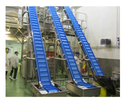
For special applications such as swan necks, the lugs can be positioned on the edges of the belt, allowing full control at the critical bend of the conveyor.
