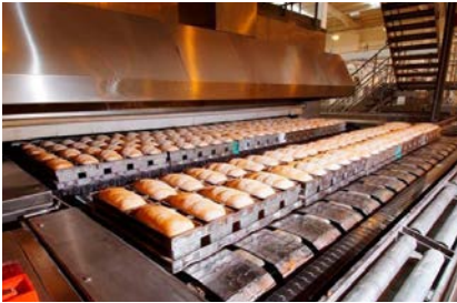
Take-off with steel chains
