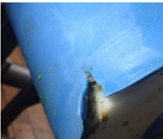
FIGURE 19: BROKEN BELT SIDE
