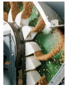
FIGURE 67: ELEVATOR BELT WITH BUCKETS
