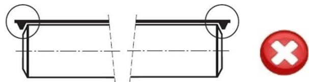
FIGURE 66: TRACKING ROPES ON THE BELT EDGES
