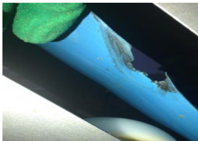
FIGURE 20: BROKEN BELT SIDE
