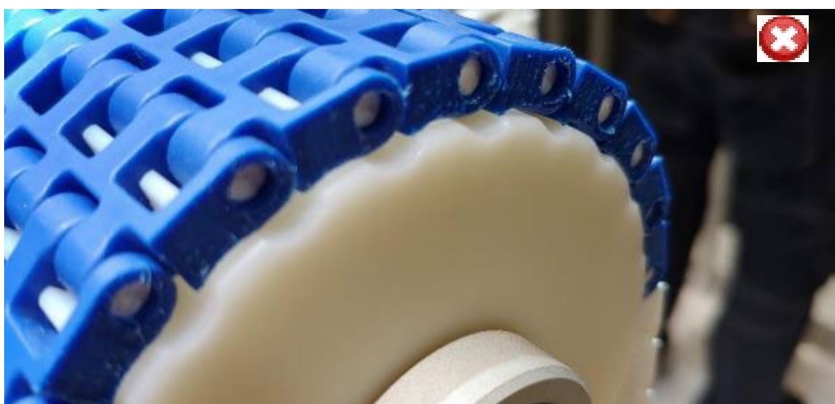
FIGURE 33: BAD FINISH OF CUT LINKS ON MODULAR BELT
