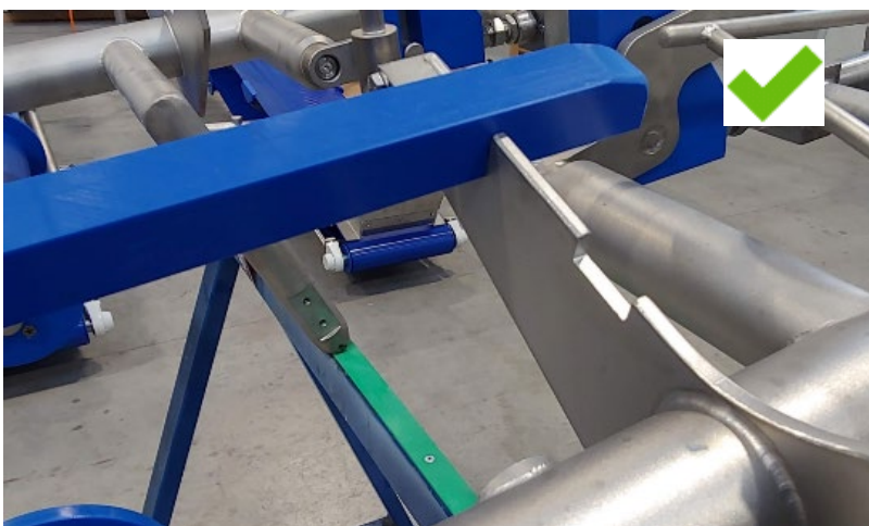
FIGURE 41: SELF-SUPPORT HYGIENIC UHMWPE GUIDE
