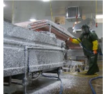
FIGURE 18: SANITATION STEP BY DETERGENT FOAM
